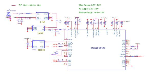
Note: The L2 inductance at V\_DCDC\_OUT is required to be 4.7 uH.
